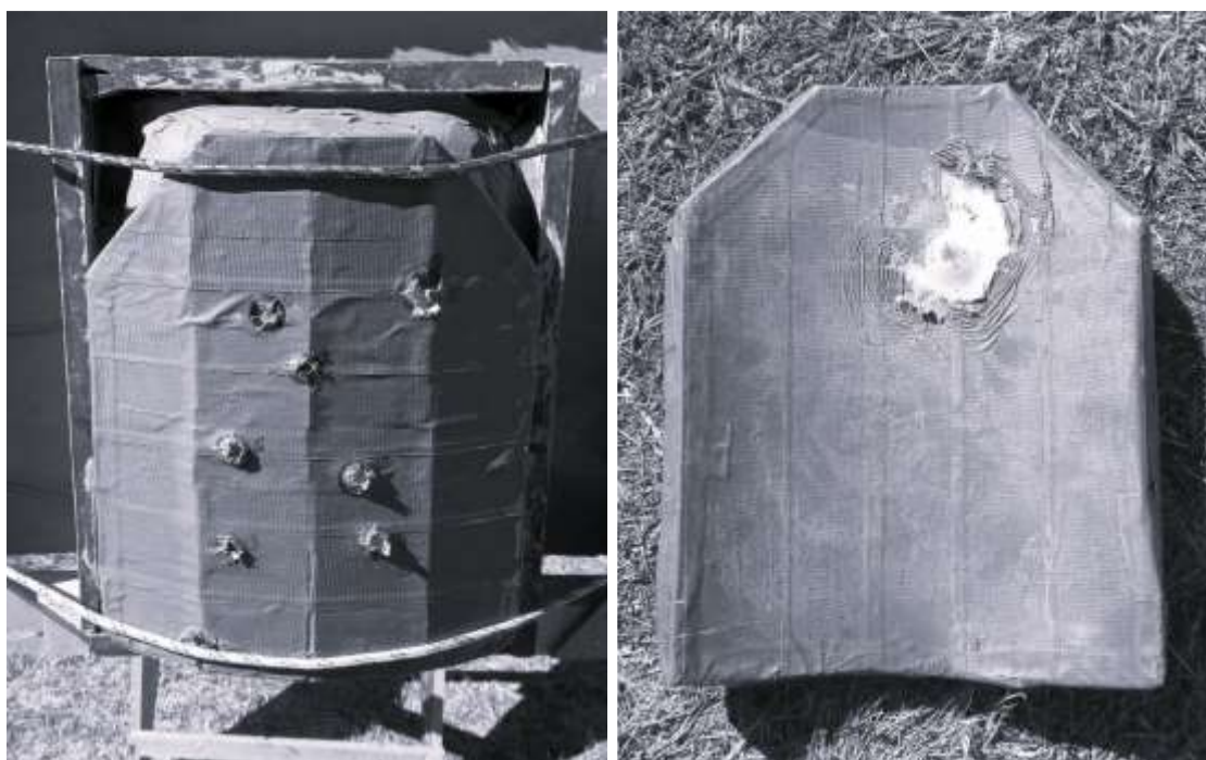
Figure 5. Plate 2 – Post testing strike and wear faces
